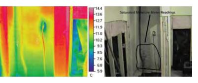
Sudden freezing conditions resulted in a discharge hose obstruction, pump failure and standing water on the floor in this finished basement. The owner removed the water and lower wall drywall according to my suggestion, but not behind the sump pump. This thermal image was taken eight days later and did not pinpoint areas of saturation identified by the moisture meter, where mould was also visible. I could not determine whether the cooler temperature was moisture or simply a cooler outside wall.
