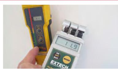
elevated moisture. This unit only senses to  $\sim 3/4$  inch depth, suggesting the drywall and insulation close to the vapour barrier was dry. The moisture meter on the right however shows 11.9 percent, which is near saturation, somewhere within 1.5 inches of the wall surface. This case demonstrates the importance of understanding the sensing range and limitations of moisture meters and the benefits of using more than one moisture meter for non-invasive moisture verification.
