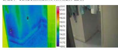
This first case shows ideal conditions for evaporation and good thermal images. Water from a burst pipe migrated to a number of apartment suites below. The leak occurred 48 hours before my visit and restoration crews had vacuumed up water the previous day, and installed air movers and dehumidifiers.
